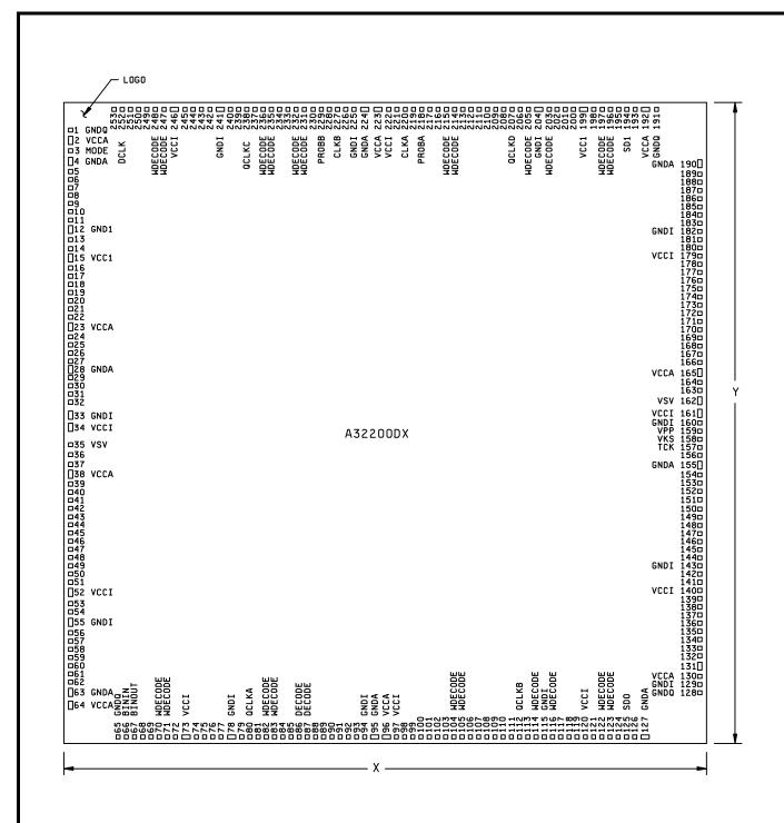
Figure A-1. Bond Pad Functions and Locations
