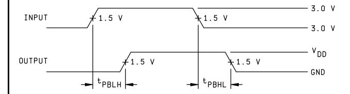
FIGURE 3. Switching test circuit and waveforms.
